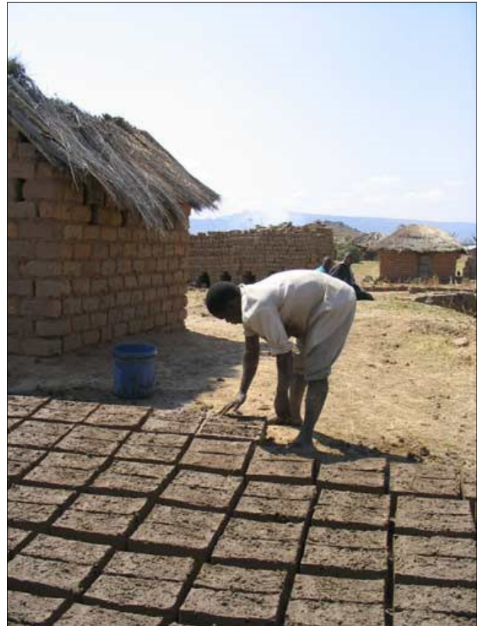
Hand-made bricks drying in the sun in Kalalasi
